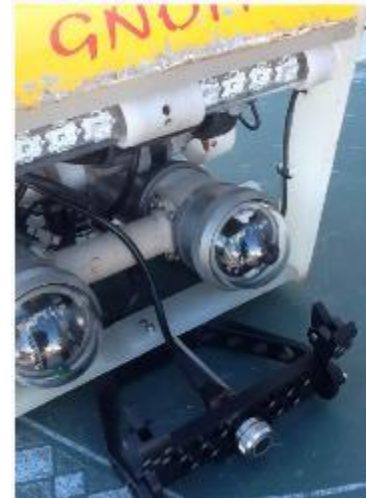
Remotely Operated Vehicle (ROV) SuperGnom PRO with ultrasonic thickness meter Cygnus onboard
